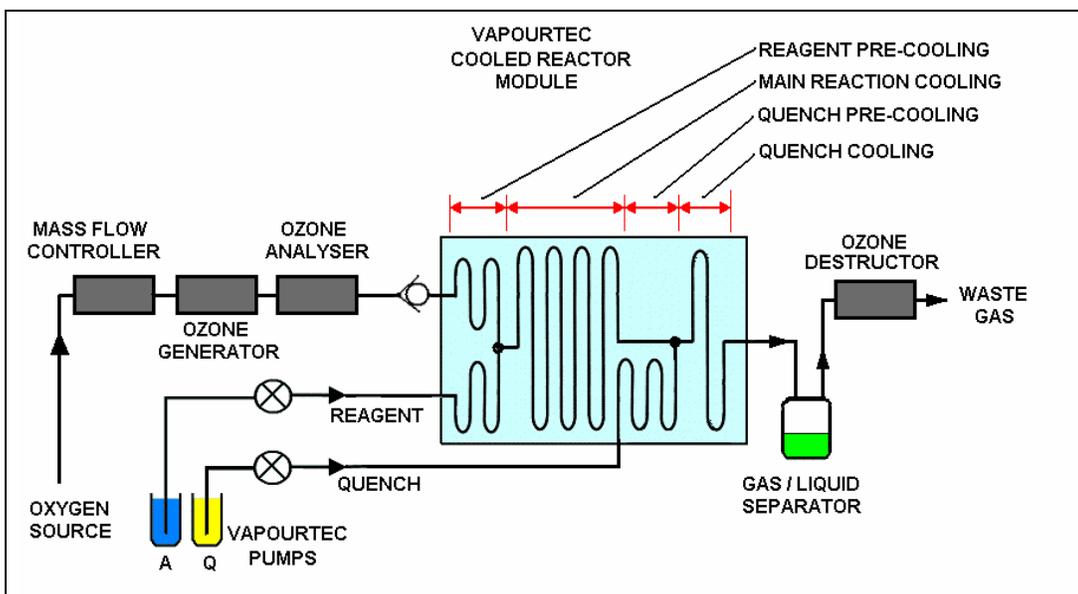
A key feature of the system is the ability to pre-cool reagents, and then to pre-cool the quench before introducing it and then have a cooled residence period while the quench takes place. This work was carried out at -10°C.
