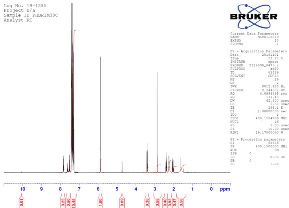
Figure 8 – NMR of 1-Phenyl-1-propanol obtain from reacting ethyl magnesium bromide with benzaldehyde at 30 °C
