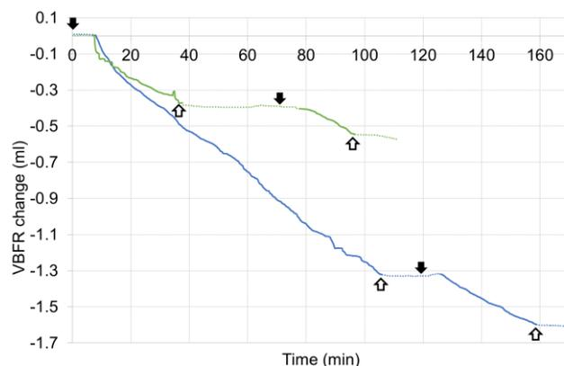
**Figure 5 – Magnesium consumption (in ml) over time when pumping a solution of bromobenzene [1 M at 0.50 ml/min (blue); 0.5 M at 0.25 ml/min (green)]. Back arrow: switch to reagent. White arrow: switch to solvent**
