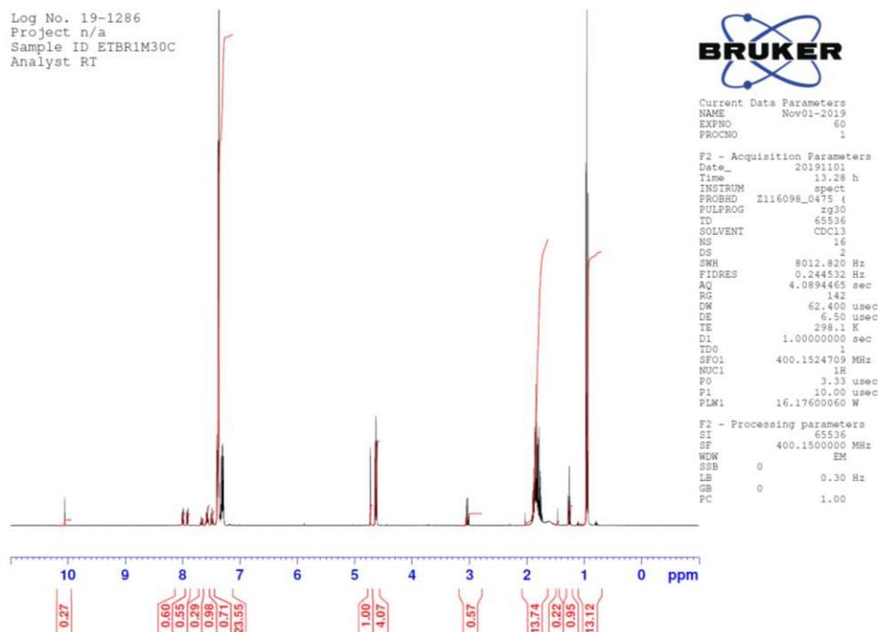
Figure 9 – NMR of diphenyl methanol obtained in flow with phenyl magnesium bromide with benzaldehyde at 30 °C in a stainless steel tubular reactor
