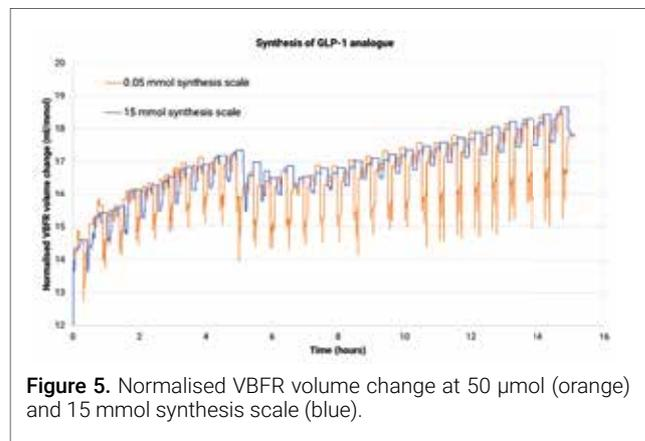
Figure 5. Normalised VBFR volume change at 50  $\mu\text{mol}$  (orange) and 15 mmol synthesis scale (blue).
