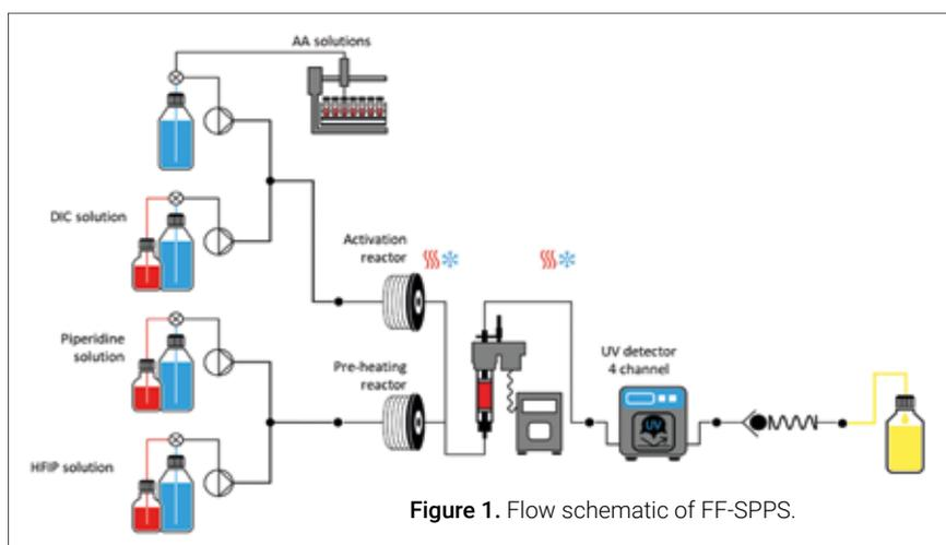
Figure 1. Flow schematic of FF-SPPS.
